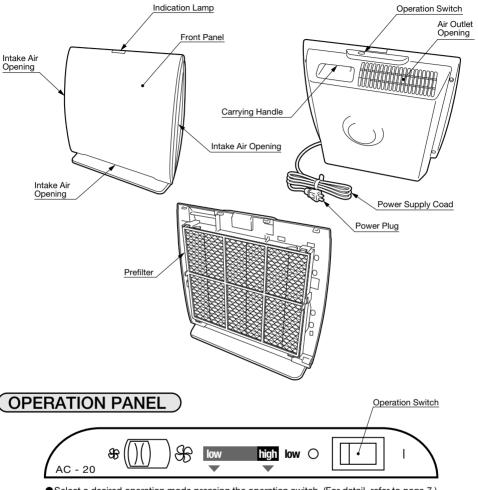
• Select a desired operation mode pressing the operation switch. (For detail, refer to page 7.)
